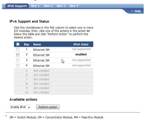
The I/O Module Configuration page initially displays the IPv6 support tab where you can view and change the IPv6 support state for each I/O module.
