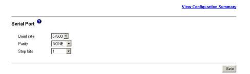
You can configure the serial port settings for baud rate, error checking parity, and the number of stop bits. Connections that are made using the advanced management-module serial port can access only the management-module CLI and the Serial over LAN (SOL) feature. See the *BladeCenter Advanced Management Module Command-Line Interface Reference Guide* for information about using the serial port.
