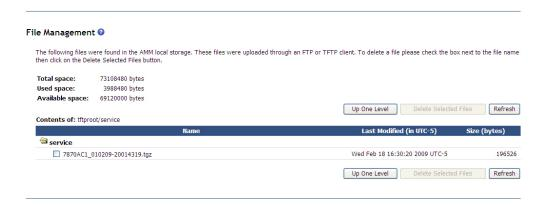
The **File Management** choice shows a list of files and available space in the advanced management module file system. You can delete files that are stored in the advanced management module. The page displays up to two levels of file
